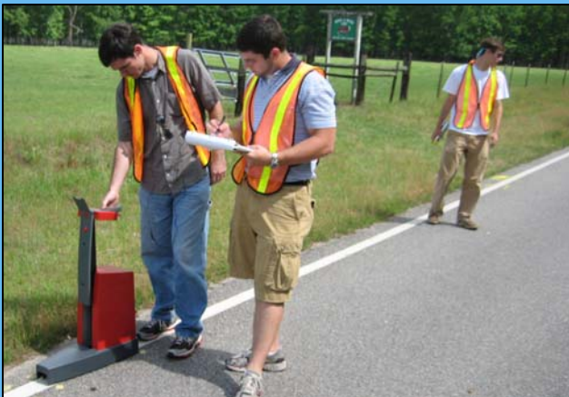
Cadets Alex Wilson, Bruce Rasmussen and Preston Dukes collect pavement retroreflectivity data on rural road near Barnwell, SC
