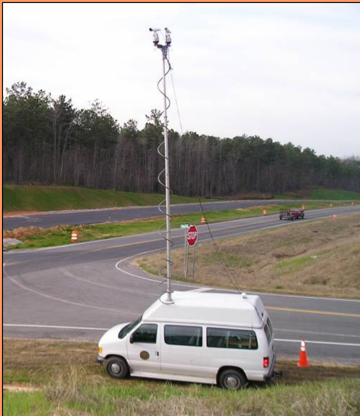
Member of Clemson's ITE Student Chapter collect data using Clemson's transportation research surveillance van.
